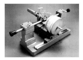
This instrument is used for accurate measurement of "Thread Plug Gauges". Gauges dimensions such as Outside diameter, Pitch diameter and Root diameter are measured with the help of this instrument. All these dimensions have a vital role in the thread plug gauges, since the accuracy and interchangeability of the component depends on the gauges used. To reduce the effect of slight errors in the micrometer screws and measuring faces, this micrometer is basically used as comparator.
