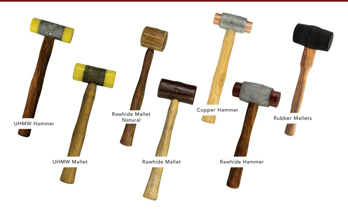
Soft faced hammers are shock absorbing hammers with ability to strike a clear blow to the work piece without damaging the surface. They have wide applications like sheet metal working, transformer manufacturing and rewinding, bearing alignments, pump and pipe fittings, smithy, carpentry, pillow block fittings, valves, automobile / aeronautical industries, power generation machineries, gear manufacturing, Foundry work, etc.
